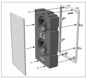
Once the frame is mounted in the wall, the speaker enclosure simply fits into the frame. Note that there is a foam anti-vibration pad affixed to the rear panel of the enclosure. This pad will eliminate any slight vibrations that occur if the back of the speaker enclosure contacts the wallboard in the wall cavity. Due to the usual slight dimensional variances in home construction, the IWCB either may or may not contact the wall surface behind it.
